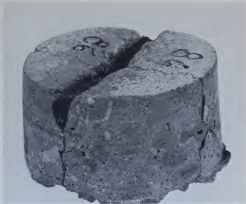
Figure 158. —Intersection of PVC plastic contraction joint-forming waterstop (longitudinal joint) with field-extruded, coal-tar extended, polysulfide canal sealant (transverse joint). Both plane weakeners developed contraction cracks; both joints are sealed. PX-D-67376.
